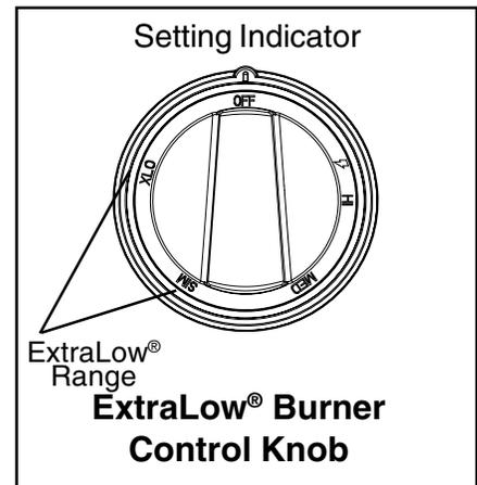
The drawing shows that the control knob has an additional range between the SIM and XLO settings. When the knob is set within this range, the flame cycles off and on. By varying the length of time the flame is off and on, the heat is reduced even further to cook delicate foods. For example, these very low settings are suitable for simmering and poaching, melting chocolate and butter, holding cooked foods at temperatures without scorching or burning, etc.
